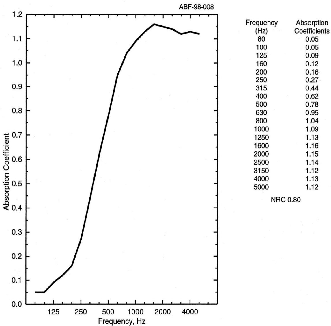
Figure 1: Sound absorption measurement of "ACPAN 6".
